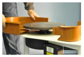
Push pan down until it is flat on the tabletop, then slide forward
