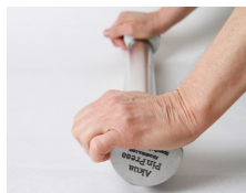
Rest the palm of your hands on the flat side of the crescent-shaped handles when printing.
